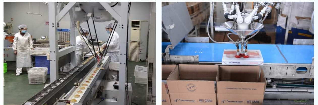
医药行业:分拣装箱整线 Pharmaceutical industry: sorting and boxing line
