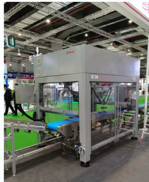
医药行业:分拣装箱整线 Pharmaceutical industry: sorting and boxing line
